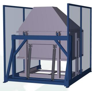
The cylinders are used to invert the top of the inverting yoke.
