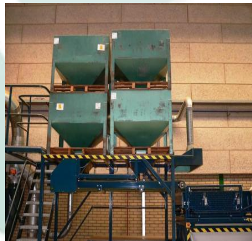
The hopper bins on top dose the seeds in the lower hopper bins. From there seeds will be transported by a belt to the flat screen sizer.
