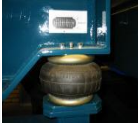
Sieve frame is mounted on four air shock absorber.
