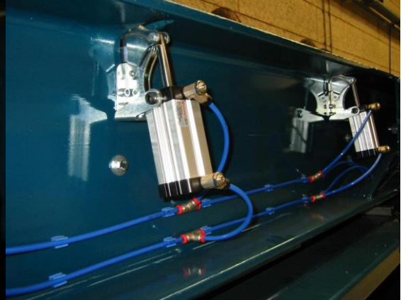
Pneumatic cylinders lock the sieves automatically in the sieve frame.
