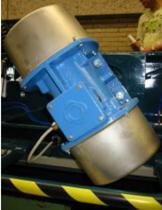
Two vibration motors are mounted on the sieve frame.
