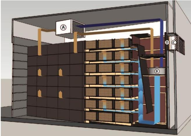
Ventilation system with humidifier and drying option.
