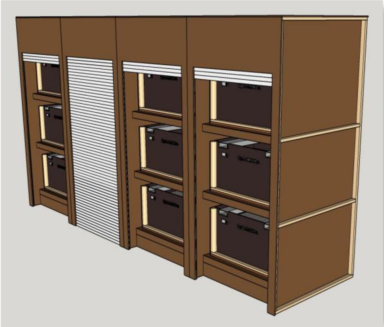
The conditioned box dryer is a closed installation with which the seed is dried to the desired moisture content at the desired air condition. This is by using dried and cooled air. The boxes are placed separately from each other in an air distribution system. Which ensures that the air is sucked through the seed. The air distribution system is located in a closed casing so that the seed can be dried regardless of the outside conditions.
